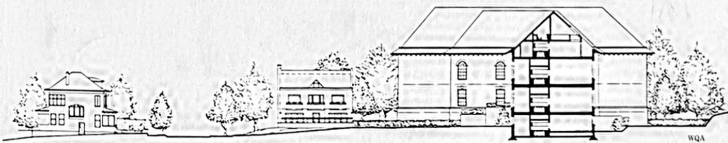
below: A cross-section view shows the two-storey high attic units and reveals the change in scale from school building to gatehouses to residences on neighboring street.
